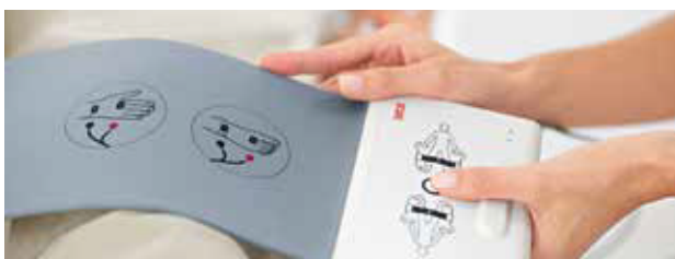
The correct placement of the electrodes is illustrated on the measuring mat. Each measurement can only begin after an automatic electrode test.
